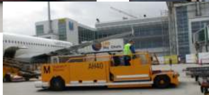
CARGO MASTER LADER TRANSPORTER CMLT 3.7-3.6 capacity 3.7 t – lifting height 3.6 m Deutz diesel D 2011 L04i, 46 kW maximum drive speed 25 km/h
