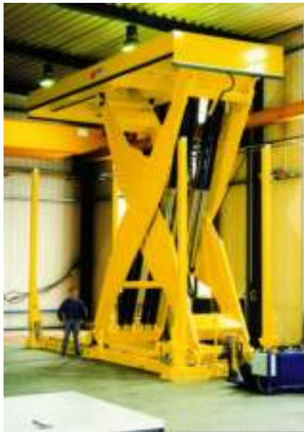
Heavy platform for feeding the process, hydraulic props for stability at levels
