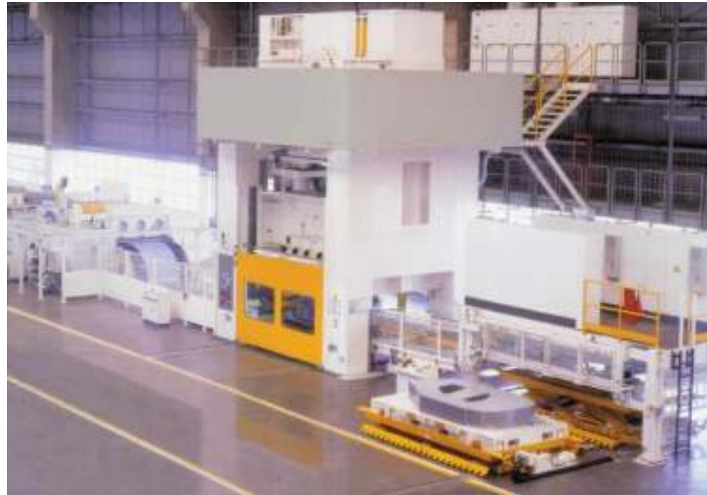
Fully integrated lift platform combination for stack movement and separation in press tool production line
