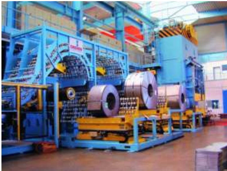
coil lift platform with conveyor to feed production line process
