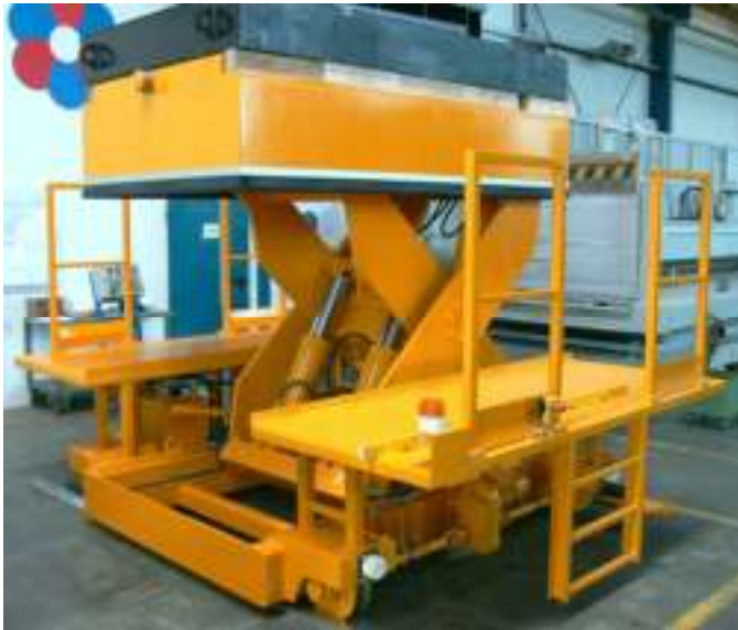
Driven assembly rig with turntable for maintenance of railway vehicles
