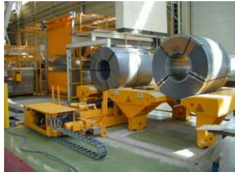
driven double coil rest equipment, safe removal and handling by driven scissor lift
