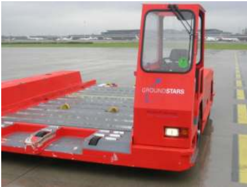
CARGO MASTER TRANSPORTER CMT7 capacity 7 t Deutz diesel TD 2011, 52 kW maximum drive speed 25 km/h
