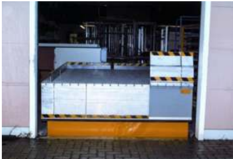
loading lift platform with roll-off protection, gap protection and aluminium loading bridge
